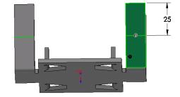
Using **Smart Dimension** add a dimension of 25mm from the top edge of the unfolded wheel arch as shown.
