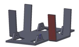
Using the **Line** command draw two horizontal lines across the inside surface of the two parallel wheel arches as shown
