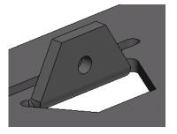
Repeat the procedure above for to bend up the final two axel holders.
